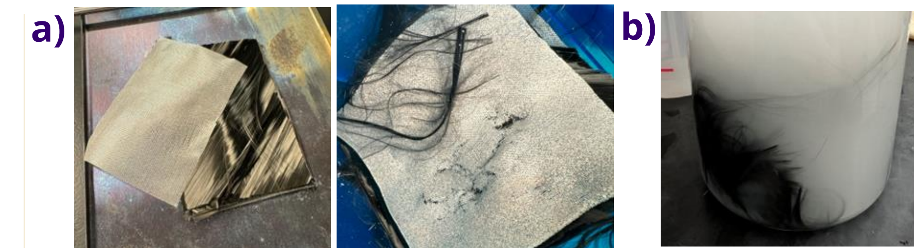
Figure 4. a) Images of the pyrolyzed coupons of 0% and 100% (left to right) removal via media blasting. b) Colloidal suspension to remove paint residue on post-pyrolysis sample.
